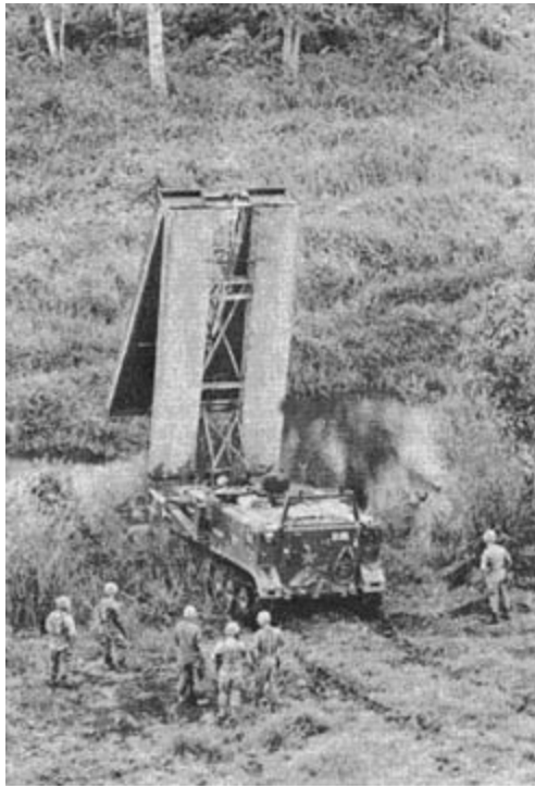
Infantrymen from Alpha Company watch the hydraulically controlled bridge lift off the armored personnel carrier to stretch across the river.
