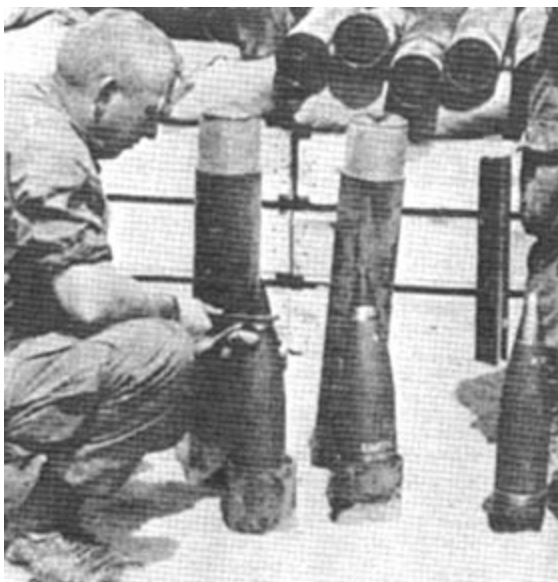
FIRE MISSION COMING - Tropic Lightning artilleryman, Corporal John Banks from Effington, Kans., of the 7th Battalion, 11th Artillery, screws a time fuse onto a 105mm howitzer round.
